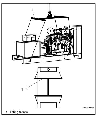
Figure 2-3 Generator Set with Lifting Fixture
